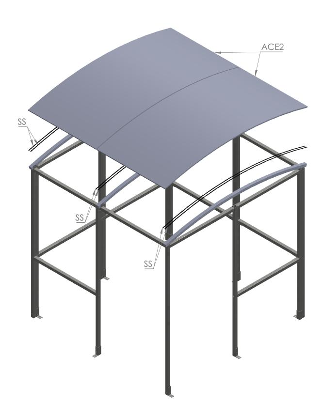
**Step 4** Apply **RC2** strips on top of the panels and use screws to secure them in place. Then clip on the **A1** angle trim to the bottom of the roof panels. Then fit the Black plastic caps on exposed nuts and bolts. Fit the square plastic end caps to any open ends of box sections.
