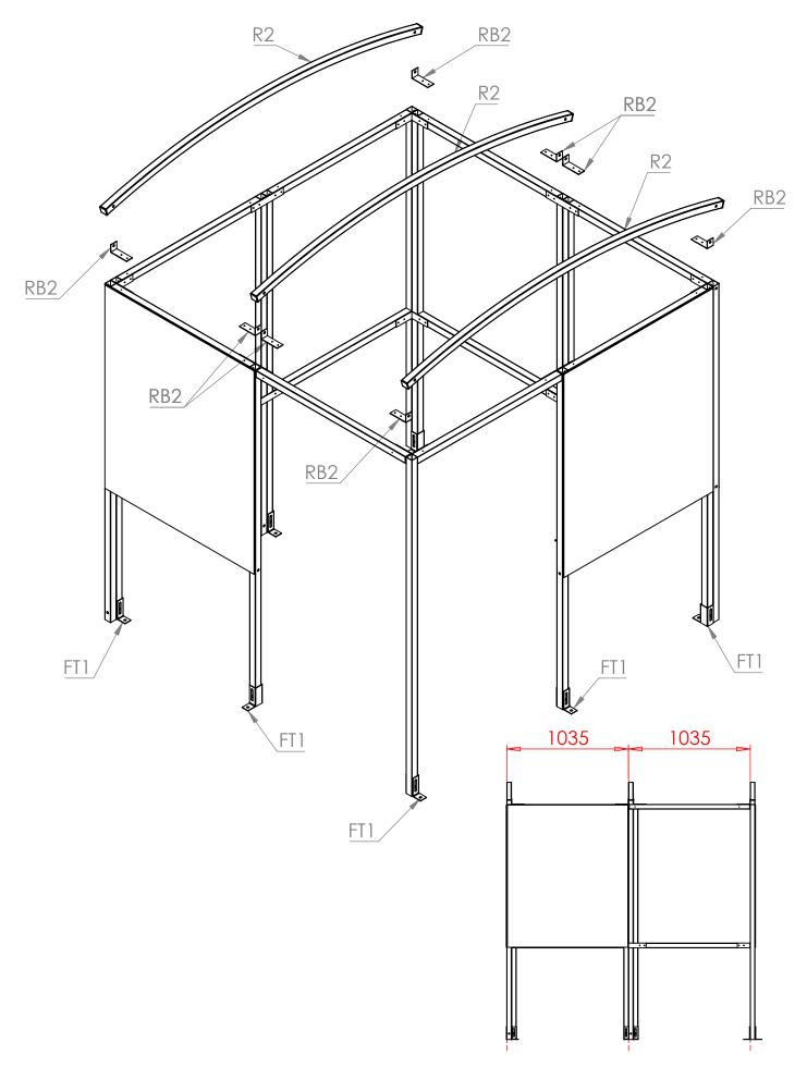
**Step 3** Apply **ss** sealing strips to the rafters (two per rafter) and line up the **ACE2** roof panels to the outside of the shelter, leaving a gap between them.
